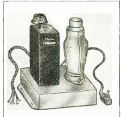
Neat and compact new Beat Frequency Oscillator gives great help in tuning in DX stations.
