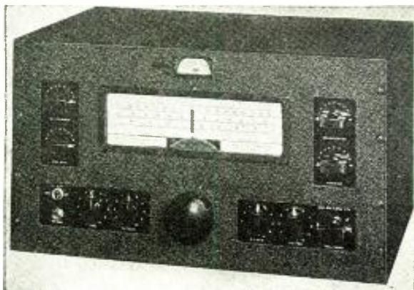
Right — Close-up view of the new 11-tube Ultra Short-Wave Receiver, showing the 3 Acorn tubes.
